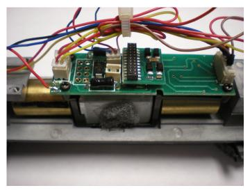
Photo shows jumper board removed Also note the Speaker Socket
